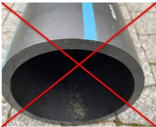
Pipe protected without the membrane (dirt visible)
