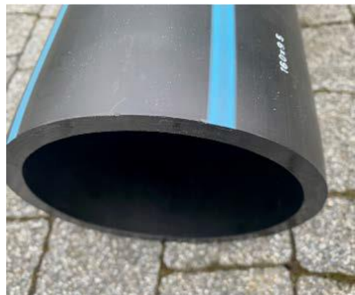
Pipe protected with the membrane (dirt not visible)
